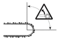
If the user does not balance out the force of the saw chain pushing backwards with his or her bodily force, there is a danger that only the tip of the saw rail will make contact with the wood and there will thus be a rebound ( Risk of rebound!).
