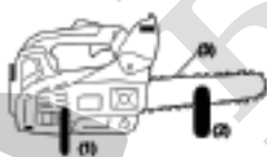
(1) muffler guard (2) guide bar (3) saw chain
