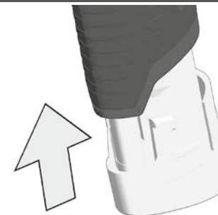
Remove the battery pack before starting any work on the machine.
