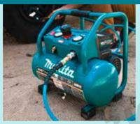
Up to 135PSI outlet pressure at 34L/min to perform a variety of tasks efficiently.
