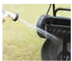
The inside of cutting deck can be washed. (Self-propelled section must not get wet with water.)
