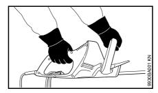
Right hand on the control handle and left hand on the loop handle.
