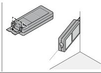
The orientation of the endpiece is automatically detected and the zero point is accordingly adjusted.
