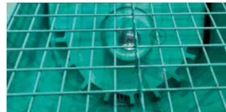
New feeding wheel design with larger cells to improve the collection of fiber materials.
