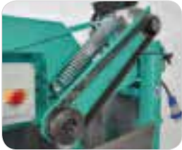
Transmission with three toothed trapezoidal belts and keyed pulleys
