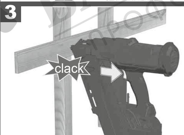
**Switch to single sequential actuation:**
