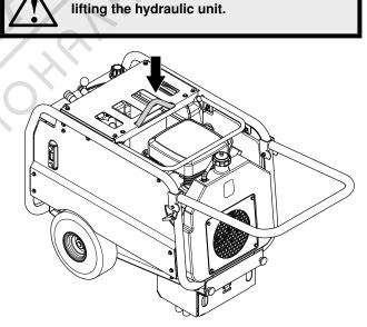
Make sure no one is standing under the hydraulic unit if it has to be moved by hand up into or off a trailer or up and down a slope.
