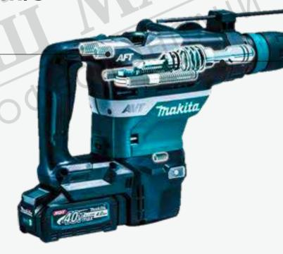
Active dynamic vibration absorber Moves in the opposite direction to The drive piston to reduce vibration
