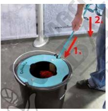
To open the bucket, you can use the shaft of the mixing paddle or another suitable tool. Stick the tool into the opening provided and push up the cover with the brushes.
