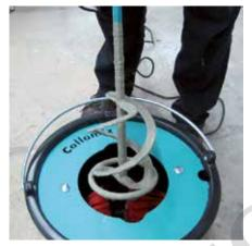
Place the dirty mixing paddle between the brushes, make the mixer rotate slowly until it is completely immersed.
