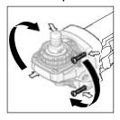
The machine head can be rotated in 90° increments. In this way, the on/off switch can be brought into a more favourable handling position for particular applications, e.g. for left-handed tool users. Completely unscrew the four screws. Rotate the machine head carefully,
