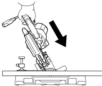
1. Loosen the lever and tilt the saw blade to set the bevel angle (Refer to the previously covered "Adjusting the bevel angle"). Be sure to retighten the lever firmly to secure the selected bevel angle safely.
