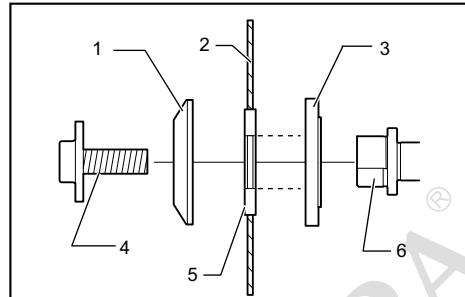
► 1. Outer flange 2. Saw blade 3. Inner flange 4. Hex socket bolt (left-handed) 5. Ring 6. Spindle
