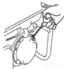
Align the notch on the starter pulley with the hole at the top of recoil starter.
