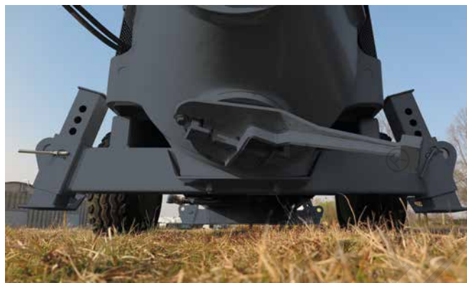
Unloading door for optimal cleaning of the hopper.
