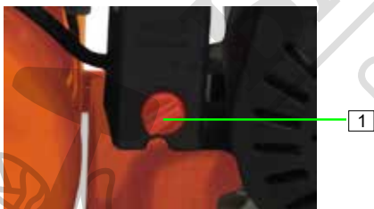
Figure 10: Switching off the air compressor
