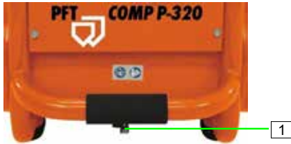
Figure 6: Closing the bleed valve
