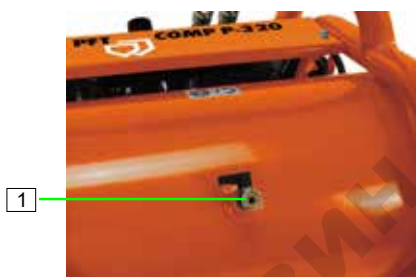
Figure 11: Open the bleed valve
