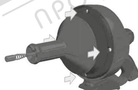
Wrap the cable carefully into the container.
